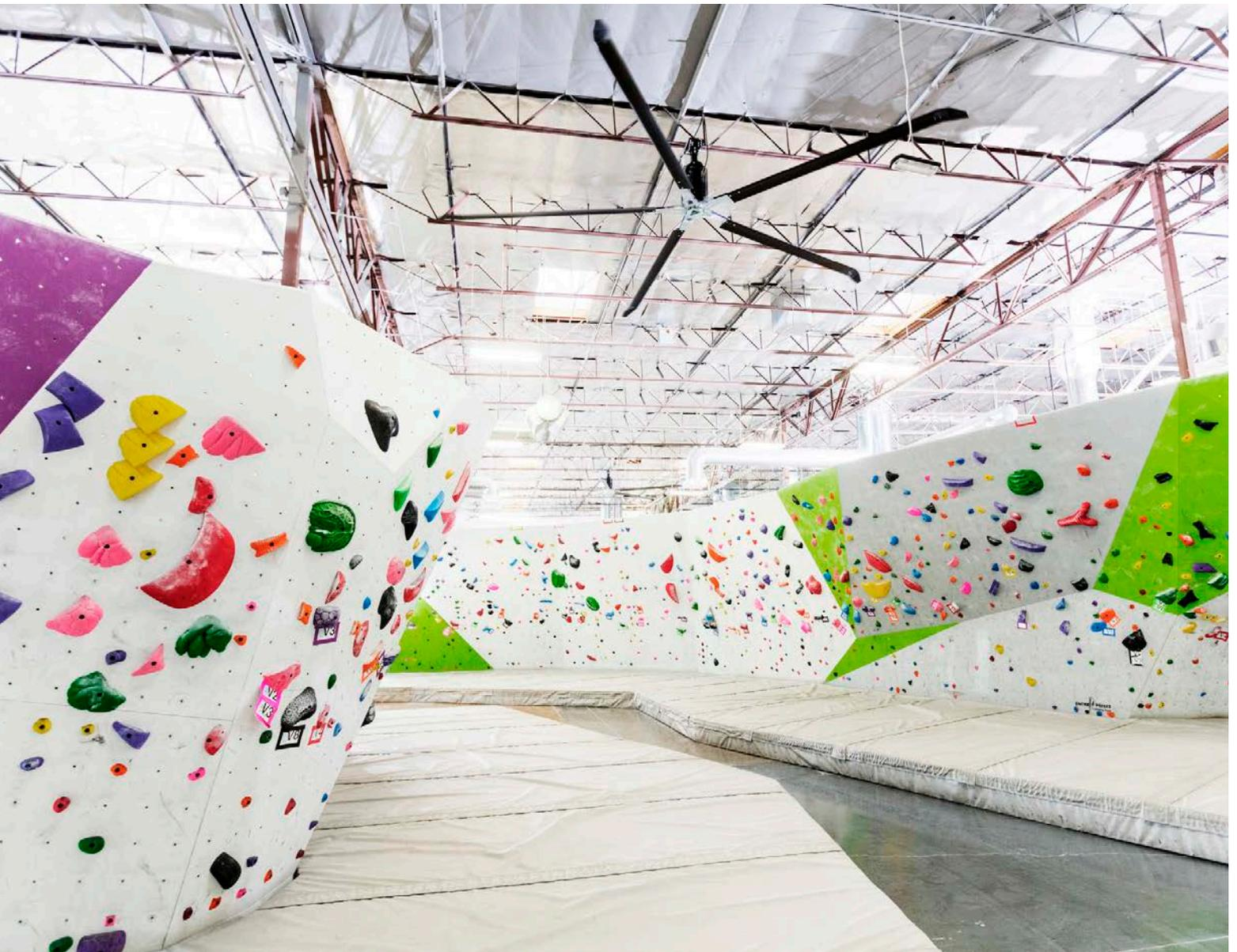
As with any large interior space—including a distribution warehouse center turned climbing and fitness center—HVAC systems only condition the air, not mix it. With the help of its two HVLS industrial fans, Origin Climbing has been able to meet its goal of providing customers a quiet, yet highly effective way of keeping them cool, comfortable and safe in what can be a brutally hot region of the U.S.
