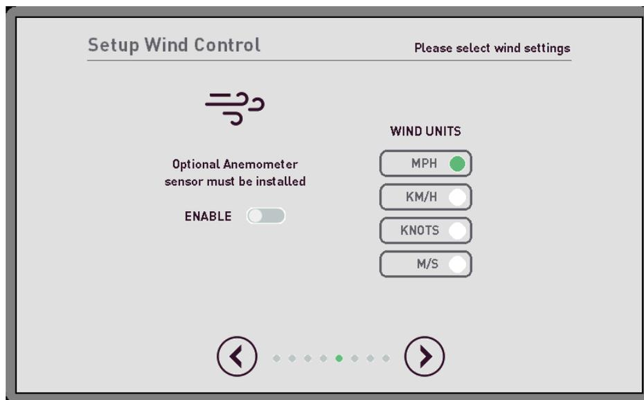
**Figure 9: Setup Wind Control Sensor Screen**
